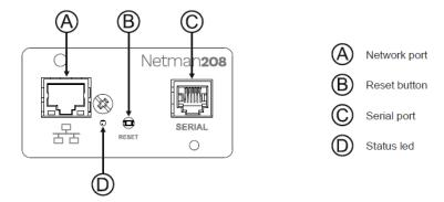
While holding the RESET button, observe the status **LED** sequence (keep the RESET button pressed):
