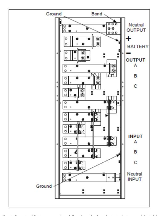
Note: For the Input, Output and Battery connections, follow the order from the top to bottom, or right to left, as described in the boxes. The label marked "N" present on the terminal identifies the neutral terminal.
