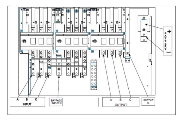
Note: For the Input, Output and Battery connections, follow the order from the top to bottom, or right to left, as described in the boxes. The label marked "N" present on the terminal identifies the neutral terminal.
