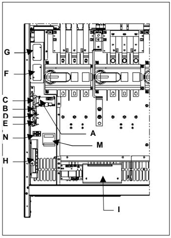
**NOTE:** Aux signals isolation board allows receiving external auxiliary contacts and keeping them isolated from the UPS internal circuits making easy connections in case of paralleling of the units.
