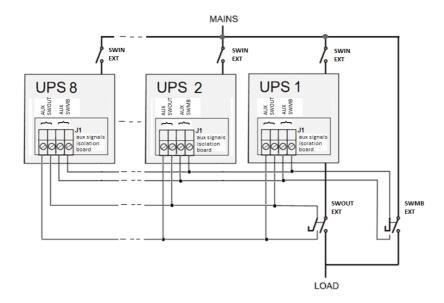
The auxiliary contacts of SWOUT EXT and SWMB EXT must be connected to terminal J1on aux signals isolation board. The purpose of this board is to isolate the internal circuits of UPS, so that, in case of parallel of UPS, one auxiliary contact of an external switch is sufficient to be acquired by all the UPS in parallel.
