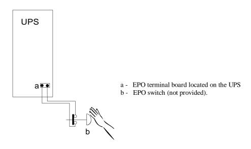
On the UPS, the jumper on the EPO terminals must be removed, and the wires from the auxiliary contact of the pushbutton must be connected in place of the jumper.
