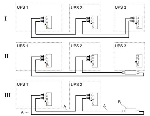
A) UPS parallel cable type RJ45 B) RJ45 female/RJ45 female shielded adaptor cable *UPS* BYPASS CABLE
