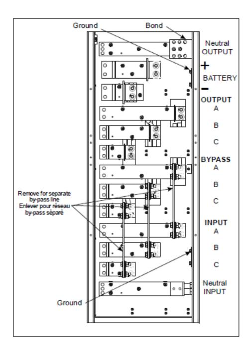
Remove the jumpers present between the BYPASS and INPUT bars.
