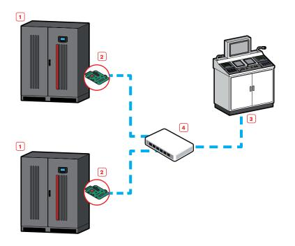
For UPS management in industrial or civil environments requiring Modbus protocol communication over Ethernet.
