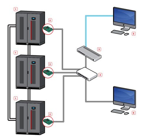
The FULL version of PowerShield<sup>3</sup> software should be used for managing setups with several UPS installed in parallel and each UPS must have a NetMan 208 board installed.
